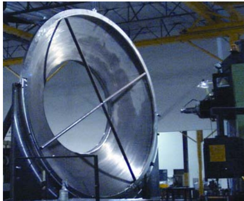
Fig 2: This 15-ft diameter dished head costs much less when made from mild steel rather than stainless steel.
