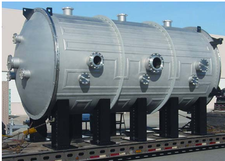
Fig 1: This large, cylindrical chamber with domed ends saves materials because the shape is very strong.
