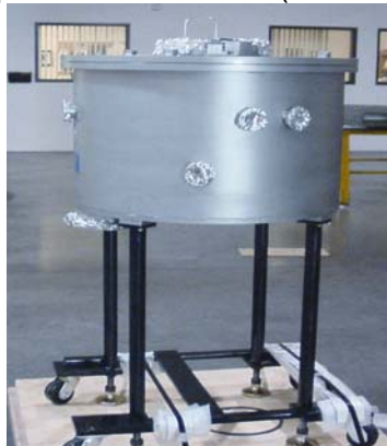
Fig 3: The painted, mild steel stand minimizes material costs.
